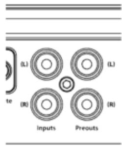
The preamp output signal by any crossover filter selected (if the input signal is full-range, the preamp output will be full-range).
