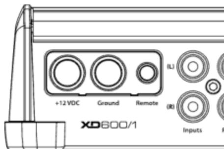
The XD600/1's “+12 VDC” and “Ground” connections are designed to accept 4 AWG power wire. **4 AWG is the required wire size for this amplifier.**
