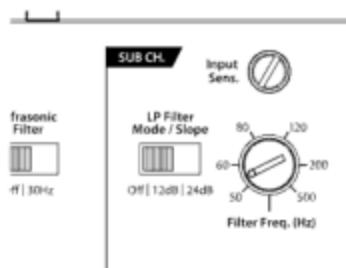
**2) LP Filter Operation:** The low-pass filter in the XD600/1 is fully variable between 50 Hz and 500 Hz via the “**Filter Freq.**” control knob and features the ability to select between a moderate “**12dB**” per octave or a steep “**24dB**” per octave slope via the “**LP Filter Mode/Slope**” switch.
