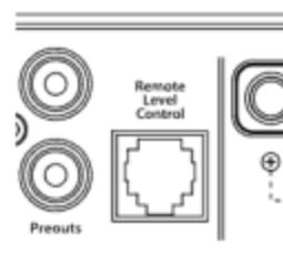
With the addition of the optional Remote Level Control (HD-RLC), you can control the subwoofer volume from the front of the vehicle.
