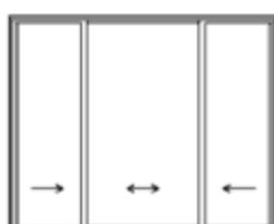
**Style #15:** To consist of three (3) full-height horizontally sliding/lift-out framed glass panels. **(Frame depth for this unit style is 2").**
