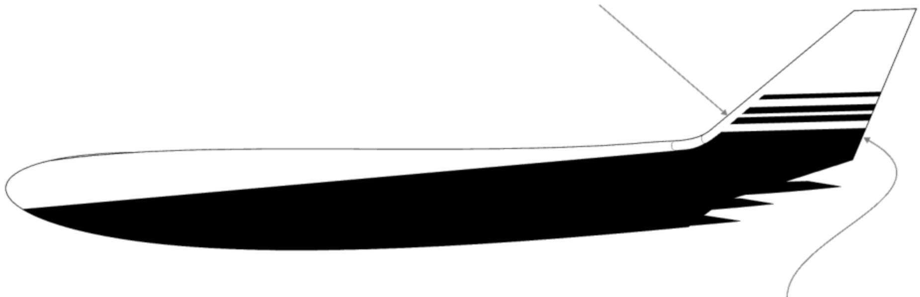
The lower inside surface of the winglet to the outboard edge of the wing is phantom gray.
