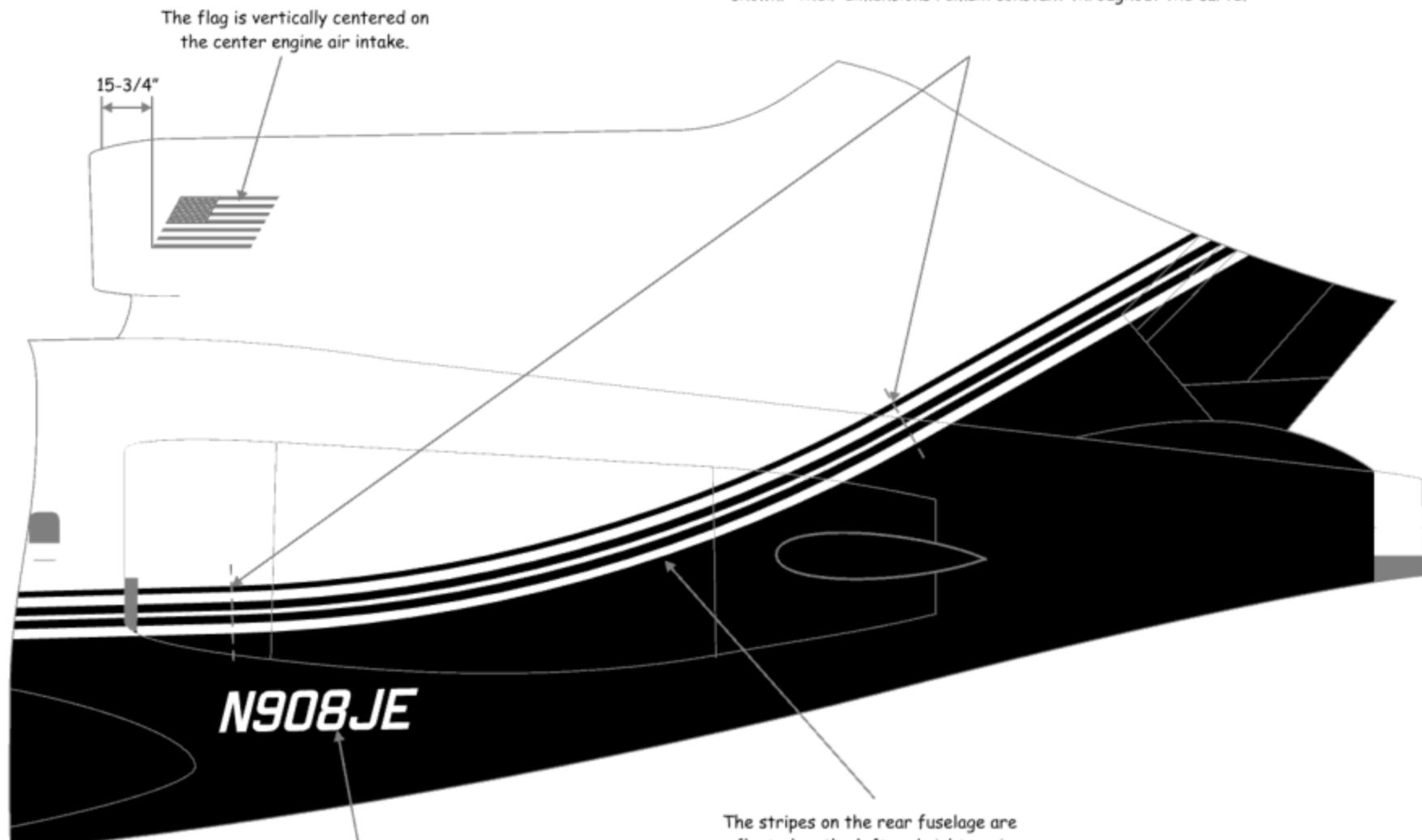
The N# consists of 12" high rounded digits, angled aft on both sides at 15 degrees. The number is rotated slightly to parallel the fuselage stripes. The number is in off white.
